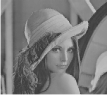
Fixed range size partition Encoding time: 5.8s. Quality: 34.39dB
